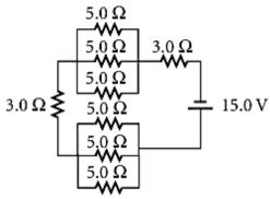
24. Determine the equivalent resistance for the circuit below.
