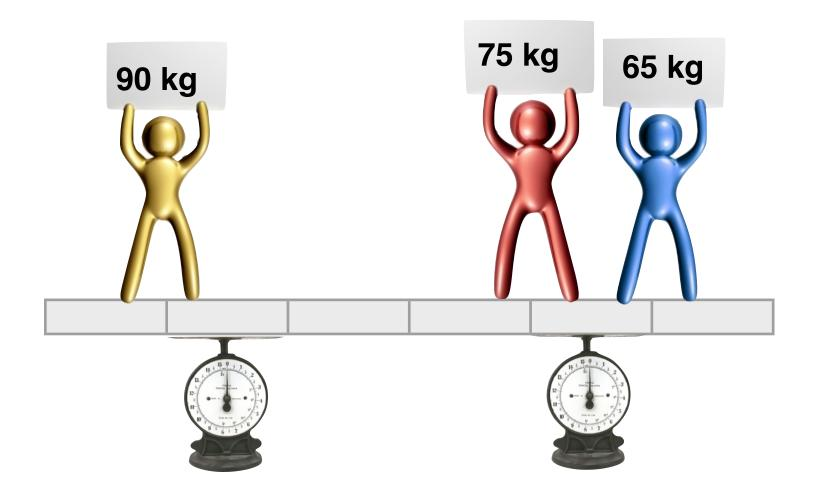
Three students with known masses stand on a 6 meter board at 1m, 4m, and 5m locations. The board has a mass of 15 kg. Two scales support the bar at 1.5m and 4.5m. **Find the force on the right and left scales**.
