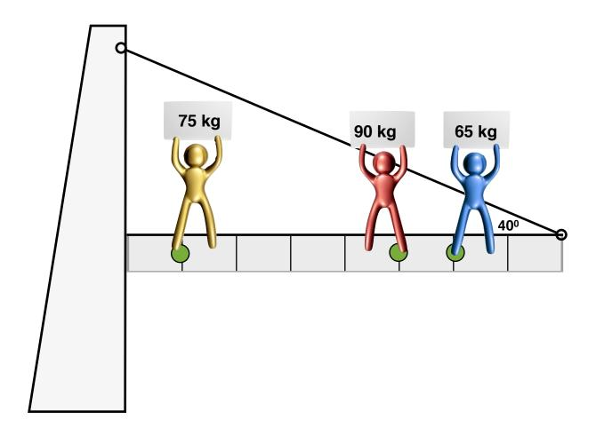
The students are on an 8m bridge at 1m, 5m, and 6m locations. The bridge has a mass of 50 kg. A support rope is tied to the end of the bridge and the wall forming angles as shown. **Find all forces**
