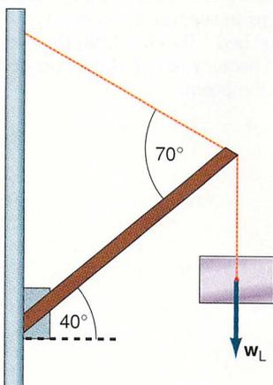
44. An 80.0-lb sign is hung on a uniform steel pole that weighs 25.0 lb, as shown in the figure. Find all the forces acting on the boom.
