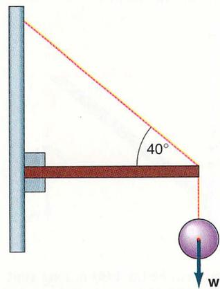
40. A horizontal, uniform boom 4.00 m long that weighs 200 N supports a load  $w_L$  of 1000 N. A guy wire that helps to support the boom, is attached 1.00 m in from the end of the boom. Find all the forces acting on the boom.
