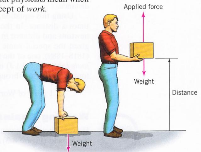
**FIGURE 8-1.** Work is done whenever a force is exerted over a distance.
