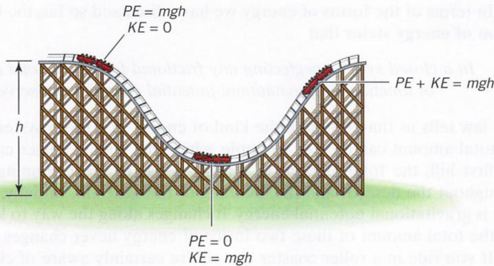
**FIGURE 8-7.** A roller coaster car has gravitational potential energy at the top of the hill and kinetic energy at the bottom of the hill. It has a mix of both kinds of energy at points in between.
