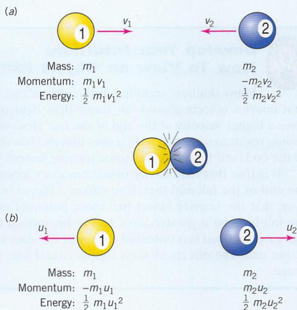
**FIGURE 8-8.** (a) A collision between two billiard balls is an example in which both momentum and energy are conserved. (b) If the two balls approach each other with the same speed before the collision, they rebound from each other with the same speed after the collision.
