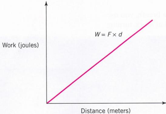
**FIGURE 8-2.** The direct relationship between work and distance illustrated in graphical form.
