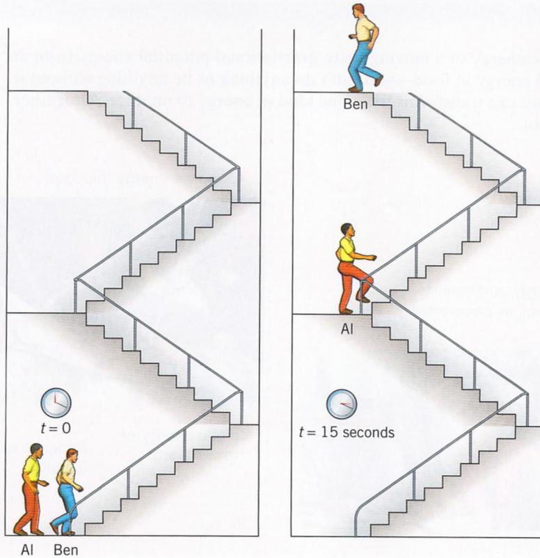
**FIGURE 8-5.** Power is the rate at which work is done, or, equivalently, the rate at which energy is expended. If Ben runs up two flights of stairs in the same time it takes Al to walk up one flight, then Ben expends twice as much power as Al.
