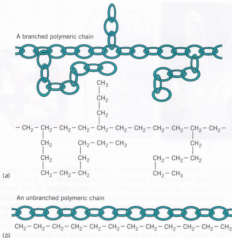
**FIGURE 9-8.** (a) Branching and (b) unbranching polymers form from small molecules, just as long chains can form individual links.
