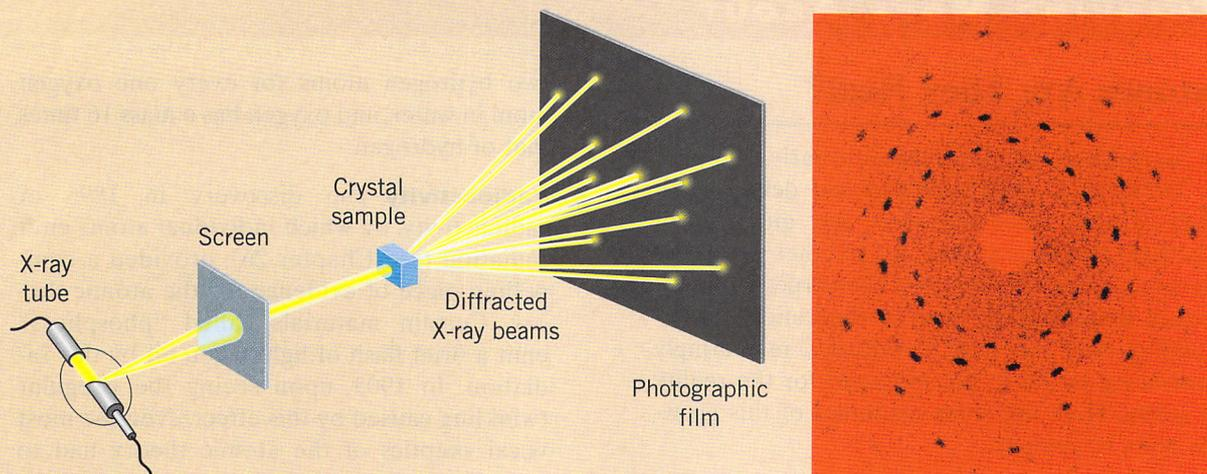
**FIGURE 9-12.** The regular atomic structure of a crystal can be revealed by the pattern of X rays that diffract off the crystal.
