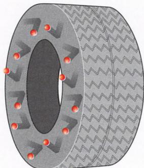
**FIGURE 9-9.** Gas molecules move constantly inside a tire. When they bounce off the inner walls of the tire, they cause an internal pressure.
