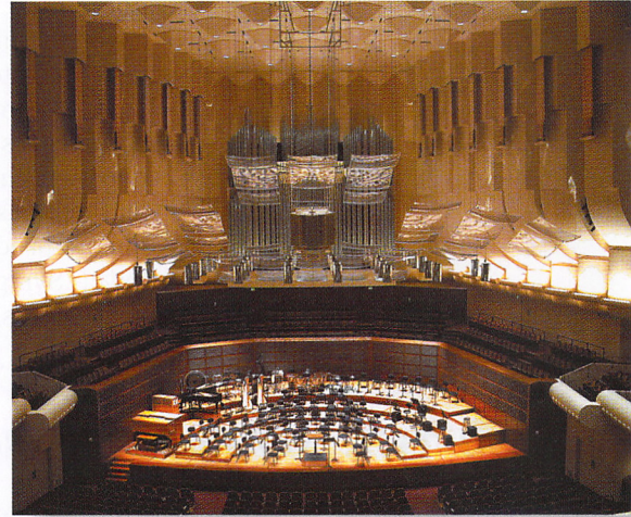
Davies Symphony Hall in San Francisco. This concert hall underwent a major renovation to improve its acoustics. Note the many sound baffles on the ceiling, hanging from the ceiling, and on the side walls.
