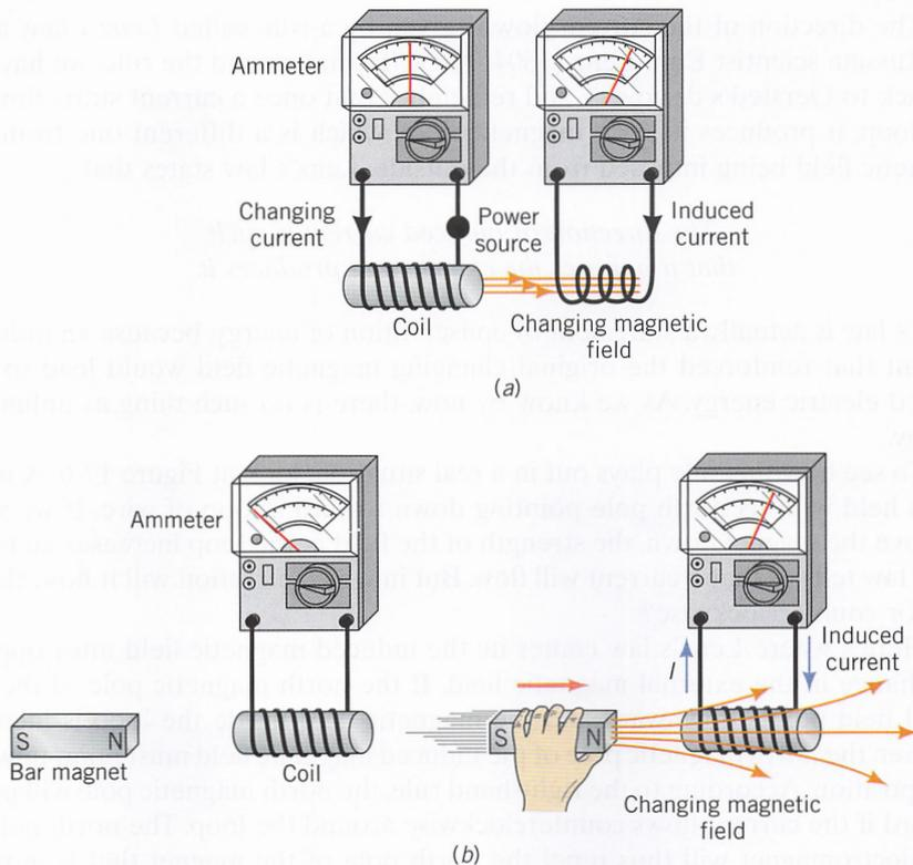
**FIGURE 17-5.** Electromagnetic induction. (a) When a changing current flows in the circuit on the left, a current is observed to flow in the circuit on the right, even though there is no battery or power source in that circuit. (b) Moving a magnet into the region of a coil of wire causes a current to flow in the circuit, even in the absence of a battery or other source of power.
