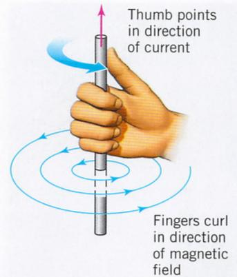
**FIGURE 17-1.** The right-hand rule states that when the thumb of the right hand points in the direction of a positive electric current, the fingers curl in the direction of the resultant magnetic field.
