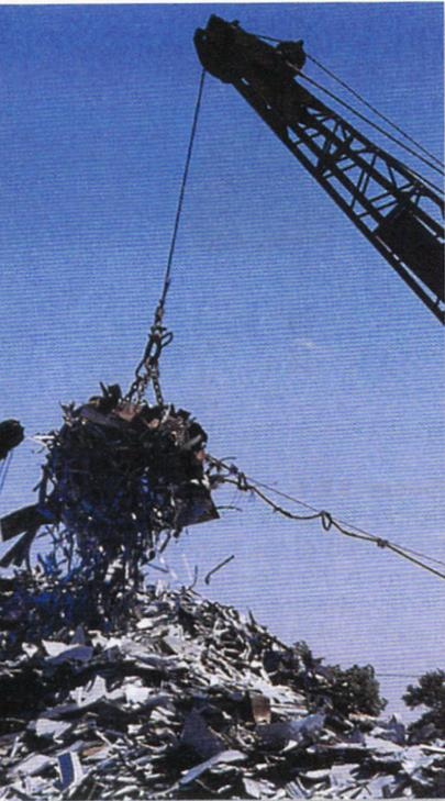
Electromagnets, which can be turned on and off, are ideal for moving scrap iron at a junkyard.
