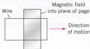
14. A rectangular piece of wire is moving to the right as shown. It passes through a region where there is a magnetic field pointing into the page, as shown (magnetic field indicated by the shaded region). When the loop of wire is in the position shown in the figure, is there an induced current in the loop? If there is an induced current, does it run clockwise or counterclockwise? Explain.
