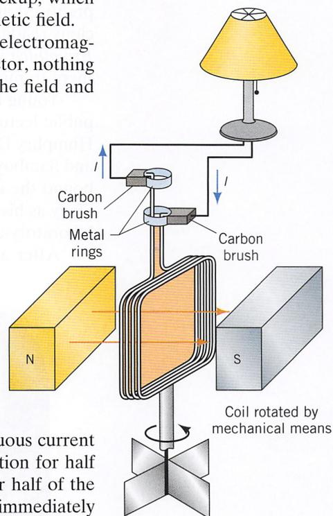
**FIGURE 17-8.** An electric generator. As long as the loop of wire rotates, the amount of magnetic field penetrating the loop changes and current flows in the wire.
