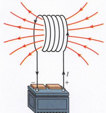
**FIGURE 17-2.** A schematic drawing of an electromagnet reveals the principal components—a loop of wire and a source of electric current. When current goes around the loop, a magnetic field forms through it.
