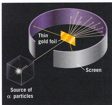
**FIGURE 21-1.** In Rutherford's experiment, a beam of alpha particles was scattered by atomic nuclei in a piece of gold foil. A lead shield protected researchers from the radiation.
