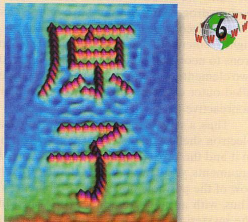
A scanning tunneling microscope image of individual iron atoms on copper forms the Japanese character for "atoms."
