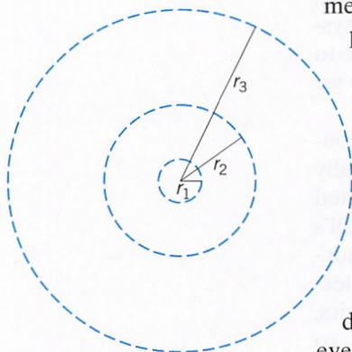
**FIGURE 21-2.** A schematic diagram of the Bohr atom showing the first three energy levels and respective distances ( $r_1$ ,  $r_2$ , and  $r_3$ ) from the nucleus.
