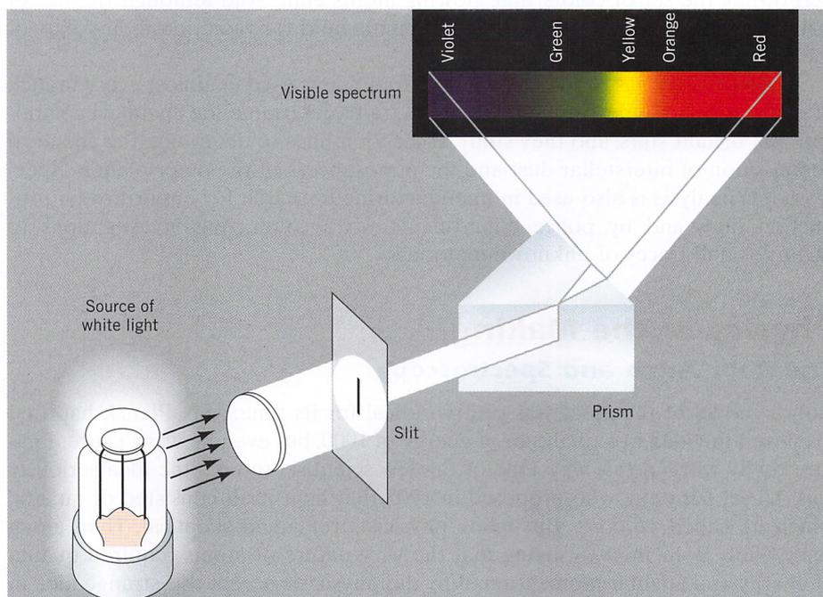
**FIGURE 21-6.** A glass prism spreads out the colors of the visible spectrum.
