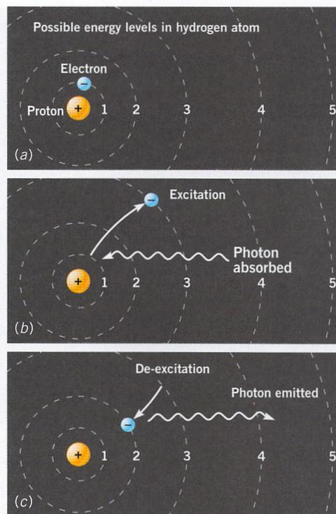
**FIGURE 21-4.** Electrons may jump between the energy levels shown in (a) and, in the process, (b) absorb or (c) emit energy in the form of a photon.
