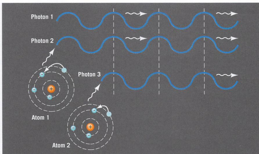
**FIGURE 21-8.** Lasers produce a beam of light when one photon stimulates the emission of other photons.
