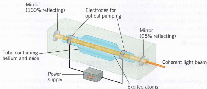
**FIGURE 21-9.** The action of a laser. Electrons in the laser’s atoms are continuously “pumped” into an excited state by an outside energy source, and the beam of coherent photons is released when the electrons return to their ground state.
