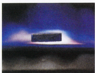
FIGURE 24-4. A magnet floats magically above a black disk made from a new high-temperature superconductor. The clouds in the background form above the cold liquid-nitrogen refrigerant.
