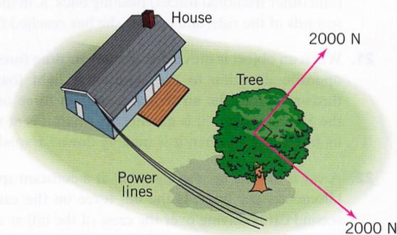
**FIGURE 4-8.** Pulling on ropes to deflect the fall of a tree. The net unbalanced force is the sum of the forces exerted on the ropes.
