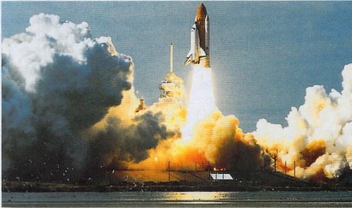
**FIGURE 4-7.** The space shuttle *Discovery* rises from its launch pad at Cape Canaveral, Florida. As hot gases accelerate violently out the rocket's engine, the shuttle experiences an equal and opposite acceleration that lifts it into orbit.
