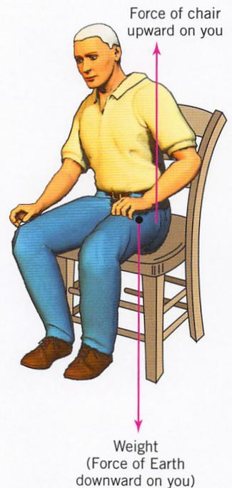
**FIGURE 4-2.** Vector diagram of a person sitting in a chair and the forces acting on him.
