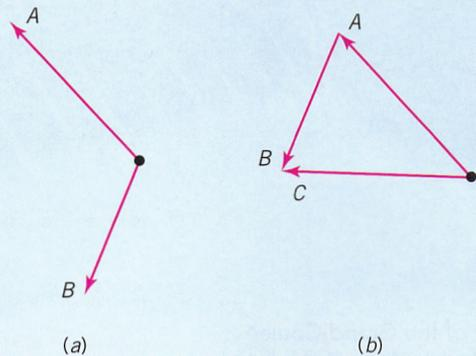
**FIGURE 4-3.** Vector addition of forces. (a) Forces *A* and *B* act on an object. (b) When vectors *A* and *B* are placed head to tail, the third side of the triangle is their sum, vector *C*.
