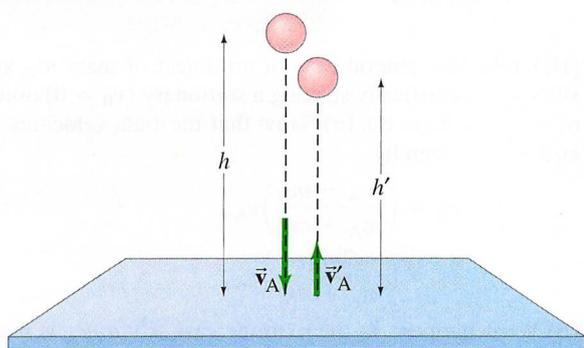
FIGURE 7-36 Problem 37. Measurement of the coefficient of restitution.
