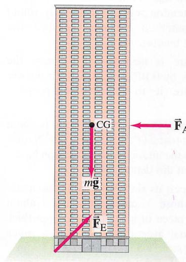
FIGURE 9–74 Forces on a building subjected to wind ( $\vec{F}_A$ ), gravity ( $m\vec{g}$ ), and the force  $\vec{F}_E$  on the building due to the Earth if the building were just about to tip. Problem 62.
