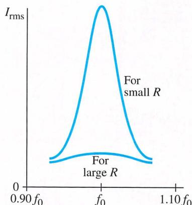
**FIGURE 21-42** Current in an  $LRC$  circuit as a function of frequency, showing resonance peak at  $f = f_0 = (1/2\pi)\sqrt{1/LC}$ .
