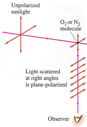
**FIGURE 24–54** Unpolarized sunlight scattered by molecules of the air. An observer at right angles sees plane-polarized light, since the component of oscillation along the line of sight emits no light along that line.
