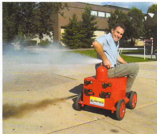
Demonstrating rocket motion with a fire extinguisher cart.
