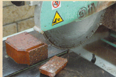
Grinding wheels with diamonds embedded in the edges are used to cut stone and metal materials.
