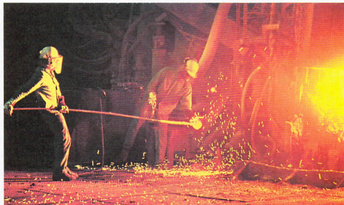
Steelworkers test a molten sample from the furnace. Because heat transfers from the hot end of the rod to the cool end by the process of conduction, the worker at the left must wear thick insulated gloves to hold the cool end of the rod.
