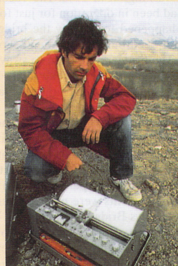
FIGURE 14-13. Two different kinds of seismic waves, longitudinal P waves and transverse S waves, travel through Earth. Geologists use a seismograph to detect these waves.
