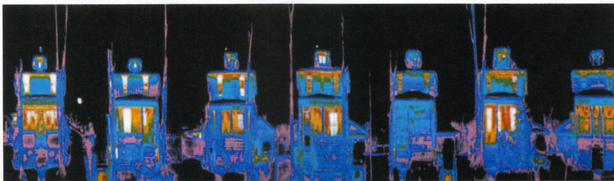
FIGURE 19-5. A photograph using infrared film reveals heat energy escaping from houses. This false-color image is coded so that white is hottest, followed by red, pink, blue, and black.
