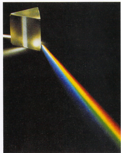
FIGURE 19-7. A glass prism separates white light into the visible spectrum.
