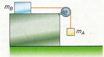
47. To determine the coefficient of static friction, the following system is set up. A mass,  $m_B = 2.50$  kg, is placed on a rough horizontal table such as in the diagram for problem 46. When mass  $m_A$  is increased to the value of 1.50 kg the system just starts into motion. Determine the coefficient of static friction.
