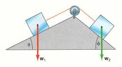
†42. In the accompanying diagram w = 50 lb, and  $\theta = 10^{\circ}$ . What must be the value of F such that w will be held in place? What happens if the angle is doubled to  $20^{\circ}$ ?
