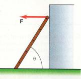
shown in the diagram. If F is equal to 50 N and  $\theta$  is equal to 63°, find the component of the force perpendicular to the ladder and the component parallel to the ladder.
