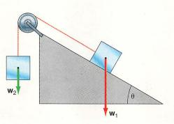
**†41.** In the accompanying diagram  $w_1 = 2$  N,  $w_2 = 5$  N, and  $\theta = 65^{\circ}$ . Find the angle  $\phi$  such that the components of the two forces parallel to the inclines are equal.
