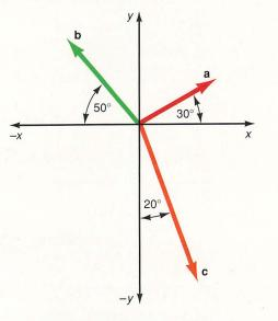
33. Find the resultant of the following three forces. The magnitudes of the forces are  $F_1 = 2.00$  N,  $F_2 = 8.00$  N, and  $F_3 = 6.00$  N.
