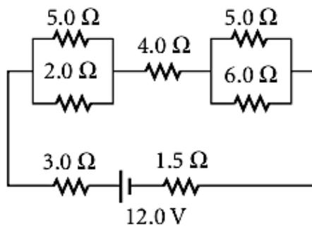
23. Determine the equivalent resistance for the circuit below.
