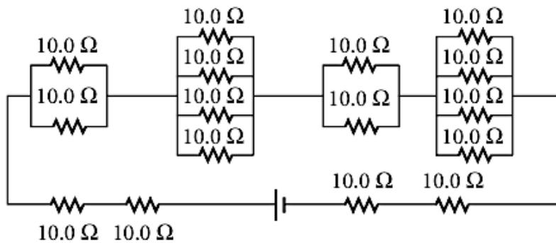
20. Determine the equivalent resistance for the circuit below.
