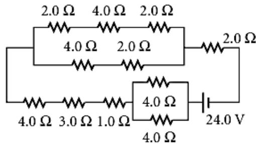
25. Determine the equivalent resistance for the circuit below.
