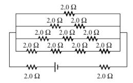
21. Determine the equivalent resistance for the circuit below.
