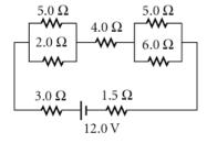
23. Determine the equivalent resistance for the circuit below.
