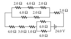
25. Determine the equivalent resistance for the circuit below.
