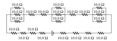
22. Determine the equivalent resistance for the circuit below.
